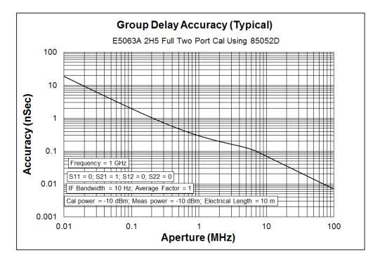
In general, the following formula can be used to determine the accuracy, in seconds, of a specific group delay measurement:  $\pm$  phase accuracy (degrees) / [360 x aperture (Hz)]
