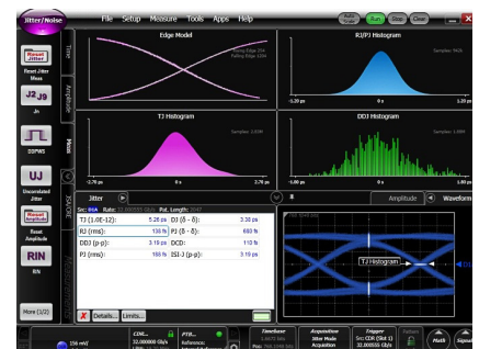
Figure 4. 32 Gb/s PRBS 211-1 showing 138 fs RJ_{rms}
