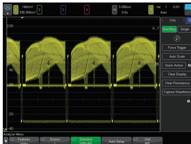
Figure 26: Triggering on 1080p HDTV signal analysis.
