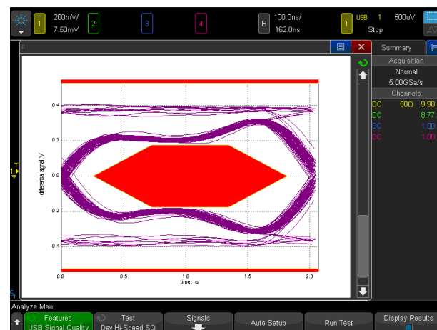
Figure 27: Perform automatic signal quality testing on USB 2.0 low-speed, full-speed, and hi-speed signals.
