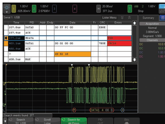
Figure 20: USB 2.0 trigger, decode and "lister" display.
