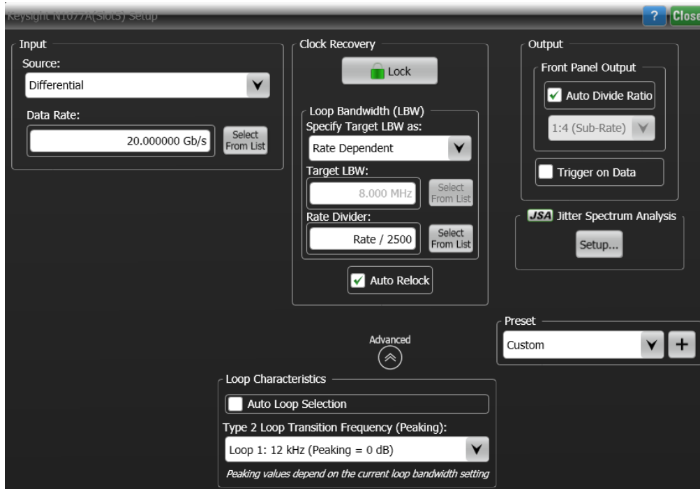
Figure 12. Easily configure the N107x clock recovery data rate, loop bandwidth, and peaking using the N1010A FlexDCA user interface running on an 86100D DCA-X mainframe or standalone PC.
