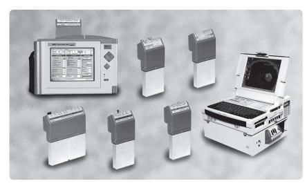
All Agilent test modules, including the Dual DS1/0 Module, can be used interchangeably with both Agilent's Service Advisor portable test tablet and Internet Advisor PC platforms. Modules plug directly into the Service Advisor tablet or Agilent's Service Advisor Undercradle, which attaches to the Internet Advisor network analyzer.
