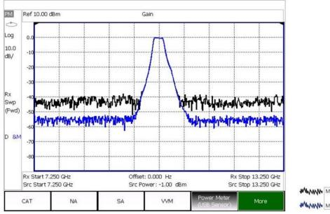
Measured using U2021XA power sensor
