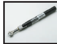
01-524, 0.8 mm-6 mm Fixed break-over torque wrench: 0.45 N*m (4 in-lb).
