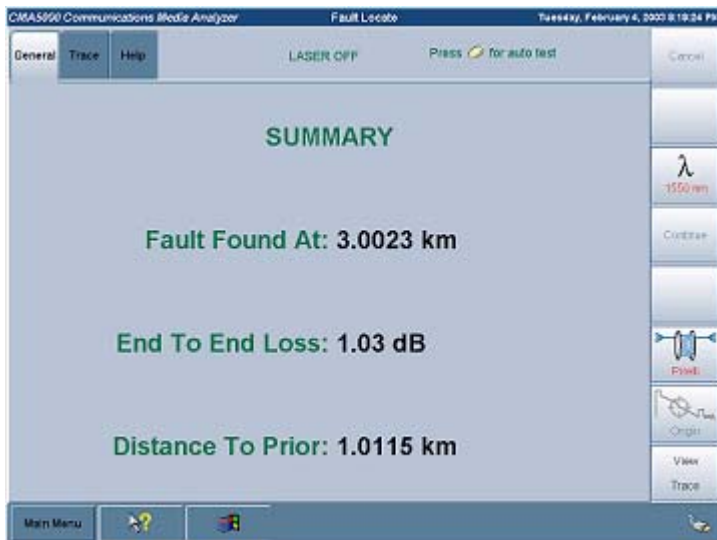
Fig.1: Fault Locate Mode - ease to read results
