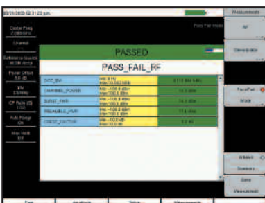
Using Master Software Tools create and download custom Fixed WiMAX Pass/Fail test sets.
