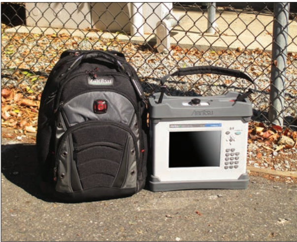
PIM Master MW82119A 40 Watts, Battery-operated
