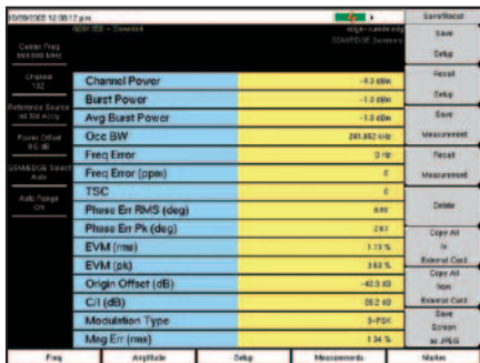
Option 41 provides a quick, table view of critical test parameters, including channel power, occupied bandwidth, phase error and EVm.
