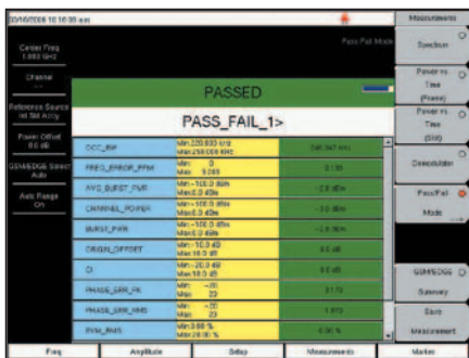
Using Master Software Tools, custom GSM/GPRS/EDGE Pass/Fail test sets can be created and downloaded in UMTS Master.
