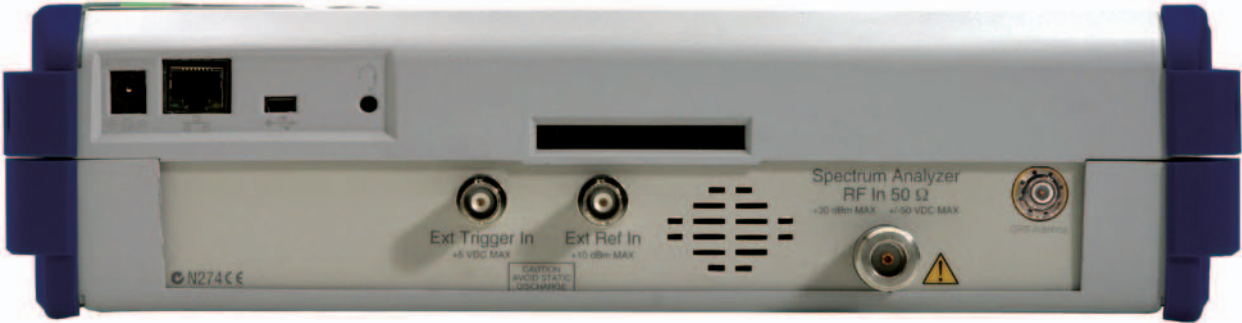
MT8220A Trigger Input, Frequency Reference Input, RF Input and GPS Connector
