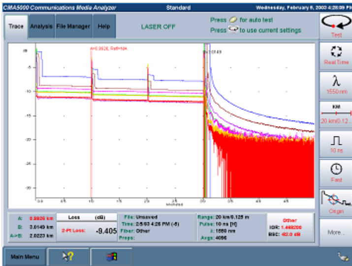
Fig.2: Classic OTDR - advanced testing
