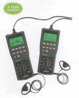
Certifies Category 5/Class D twisted pair cabling. Autotest suite includes Power Sum NEXT, Attenuation, Power Sum ACR, Length, WireMap, Propagation Delay, Delay Skew and headroom margin. Operates from AA cells, AC/mains adapter, or optional NiMH battery pack. Includes hard carrying case.
