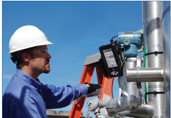
The magnetic hanger accessory allows you to attach the Trex unit to a pipe, freeing up your hands for other work.
