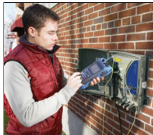
Step 1: Connect the launch fiber
