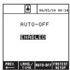
Save battery operating time. The Auto-Off function shuts the unit down after 15 minutes of inactivity.
