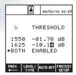
Configure Pass/Fail thresholds for each wavelength. If results exceed thresholds, an alarm and a highlighted value on the screen will notify you.
