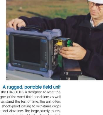
rigors of the worst field conditions as well as stand the test of time. The unit offers shock-proof casing to withstand drops and vibrations. The large, sturdy touchscreen is resistant to shock, water, dust, and common chemicals. The outershell is waterproof with sealed joints, and door panels protect connectors, ports, and the floppy disk drive. The FTB-300 UTS also complies to all industry standards.
