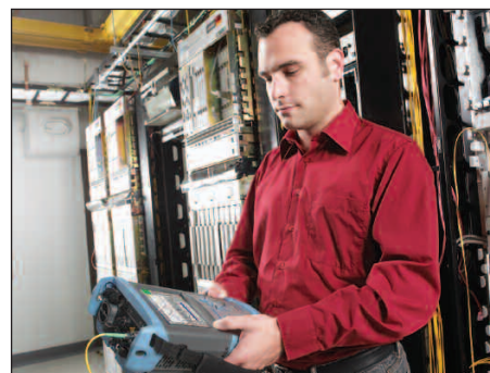
The industry's most compact eight-wavelength portable test solution, EXFO's FTB-7400E OTDR enables fast troubleshooting through CWDM-based multiplexers and demultiplexers.
