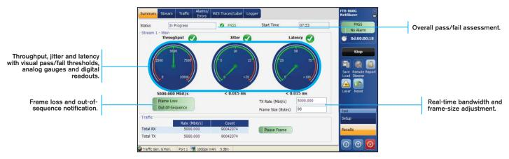
The analog gauges are lined with **Green** and **Red** layers to represent the expected thresholds.
