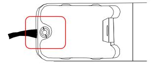
**3.** With a flat-head screwdriver, press down on the small silver ball until the head of the screwdriver fits into the small grooves on each side of the screw.
