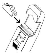
**3.** Place the fiber gently in the alignment groove of the adapter head.
