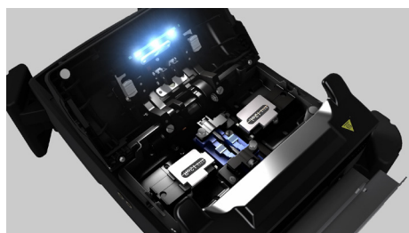
3 LED's provide a bright operation environment
