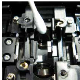
DETACHABLE V-GROOVE FOR EASY CLEANING
