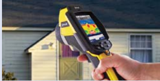
Infrared cameras quickly locate moisture related problems
