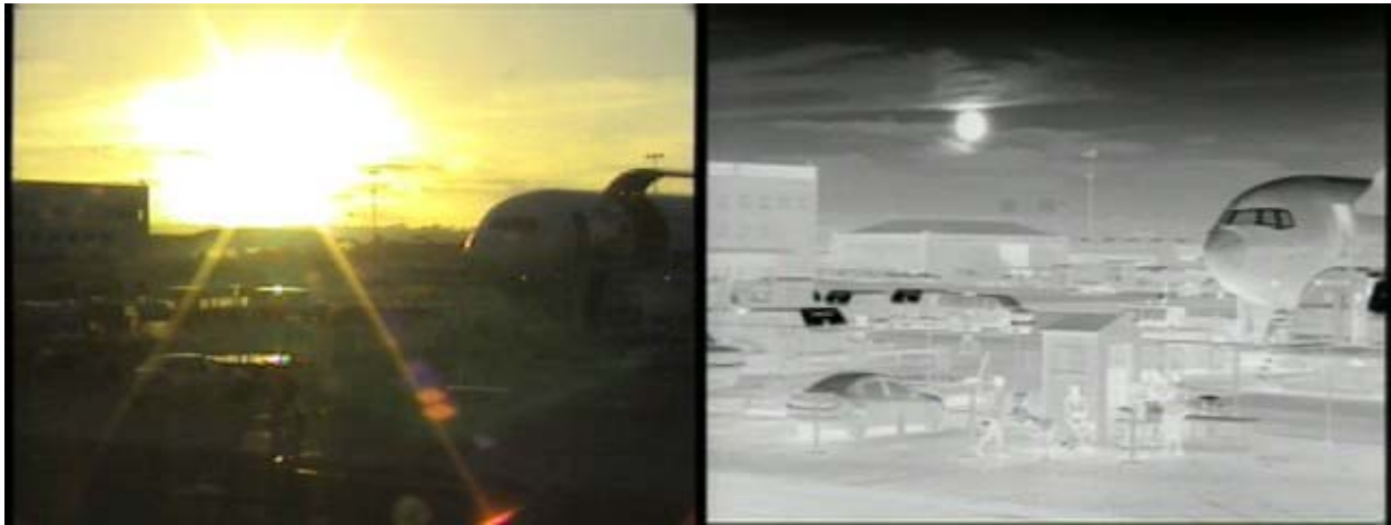
Figure 17: Backlit daylight camera on left; thermal image on right
