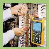
Quickly check the control signal from the digital board without even touching a button. Triggering, amplitude and timing are automatically set to provide a stable display of even a complex digital control signal.
