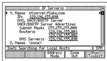
The LANMeter will check for the availability of the router, and report if the router is not responding.
