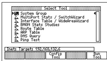
Use **Interface Table** to obtain a list of interfaces on a host, and Display Statistics for more detail about a selected interface. The LANMeter supports most LAN and WAN interface MIBs, such as 10/100 Mbps Ethernet, Token Ring, and FDDI. (For information retrieved WAN interfaces, see the WideAreaWizard Option section on page 11)
