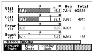
The Token Ring results screen shows utilization and soft errors in numeric and bar graph formats, and other key frames as average, maximum, and total numerical values.
