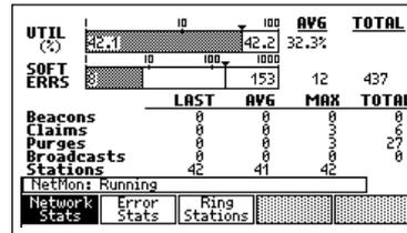
This test may be configured to store log files of results captured at various time intervals from 24 minutes to 7 days. Log files are exported as comma-separated variable (CSV) files for detail analysis and report generation.
