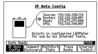
The Auto Configure feature can make use of Dynamic Host Configuration Protocol (DHCP) or BOOTP servers. The function can also be used to verify the connection to the DHCP or BOOTP server.
