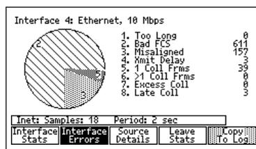
For devices supporting RMON, the LANMeter could retrieve utilization and error information from the RMON MIB using the **RMON stats studies**.
