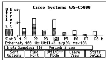
The SwitchWizard Option will display information for any type of SNMP monitored port: Ethernet, Token Ring, Serial Links, FDDI, even very high speed switch backplanes.
