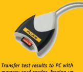
Transfer test results to PC with memory card reader, freeing up your DSP-4100 for testing
