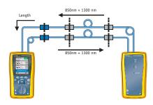
Unlike competitive fiber adapters which measure length and *two* loss measurements per Autotest, DTX is the only fiber test solution that measures length and *four* loss measurements per Autotest – all in about 12 seconds. With DTX Fiber Modules, you can speed through fiber testing five times faster than the competition.
