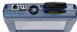
Top Interfaces – 10/100/Gigabit twisted pair copper port, Gigabit Fiber SFP transceiver, CompactFlash® memory card and 802.11a/b/g WLAN adapter.
