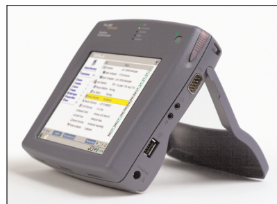
Side Interfaces – RS-232C serial port, USB port, microphone and headphone jacks, Kensington lock (opposite side).
