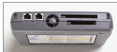
Top Interfaces – 10/100/Gigabit port, wire map port, CompactFlash® and PCMCIA slots.
