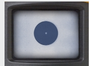
FT400 FiberInspector (400x) shows higher magnification image of singlemode fiber end-face
