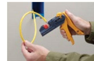
3. Insert jack in JackRapid front first with IDC slots facing blades of JackRapid.
