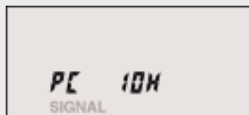
Figure 4. 10 Base-T signal detected, wired to PC.
