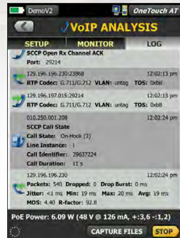
Figure 9. Inline VoIP analysis simplifies troubleshooting of desktop VoIP problems in real-time without TAPs or switch mirror ports
