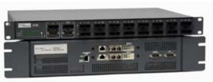
OptiView Link Analyzer (OPV-LA) with a 8-port Fiber Tap (FTAP-8M)
