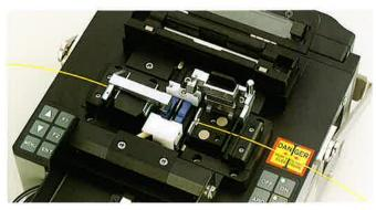
The careful ergonomic design of the FSM-15S includes the use of large, deep precision V-grooves which ensure that it is easy to load the fibers into the splicer in field conditions.
