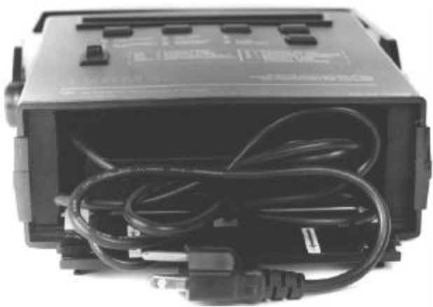
Figure 3. Bottom panel of the Test Kit, showing the 120 Vac power cord and the battery-storage area.
