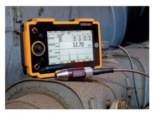
The DMS Go from GE's Inspection Technologies business is a high-end thickness gauge which combines an innovative, easy-to-use user interface, powerful data management and an ability to provide accurate, reliable and comprehensive thickness inspection data. It is ideally suited for a wide range of applications including measuring for corrosion in the oil and gas sector and in power generation.
