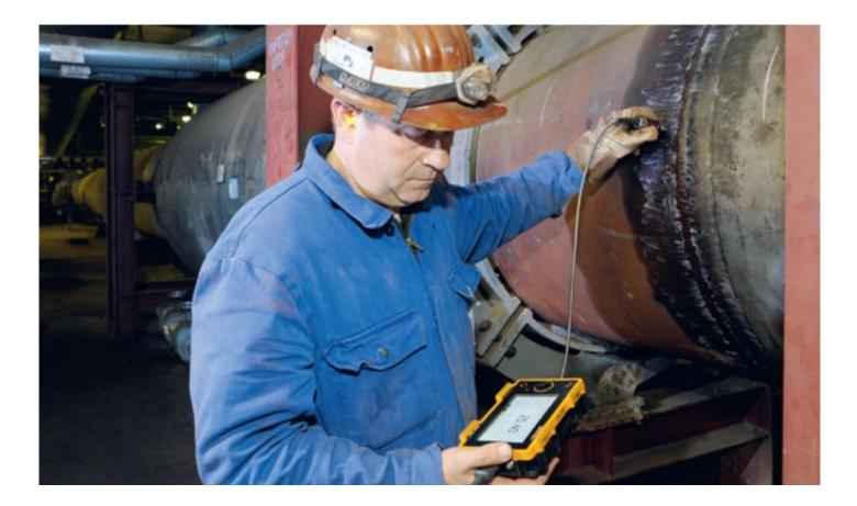
The DMS Go high-end thickness gauge is suited for thickness measurement in a wide variety of applications and especially for corrosion measurement/monitoring, even at high temperatures and on coated parts.
