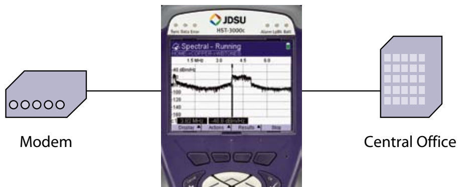
Example of HST-3000 performing Spectral Monitoring
