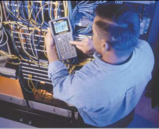
The FIBERTEK fiber accessory for the LANTEK 6 and 7 is the perfect solution for certifying or troubleshooting fiber backbones and fiber to the desktop installations in single building and campus environments. FIBERTEK measures signal loss, length, and delay over Multimode and Singlemode fiber. In addition dual wavelength, bi-directional testing is enabled by having both a transmitter and receiver in each adapter.
