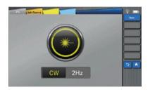
VFL allows for finding direct fault locations in fiber test dead zones or performing fiber core calibration in multi-fiber cables.
