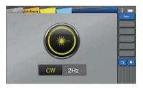
VFL allows for finding direct fault locations in fiber test dead zones or performing fiber core calibration in multi-fiber cables.
