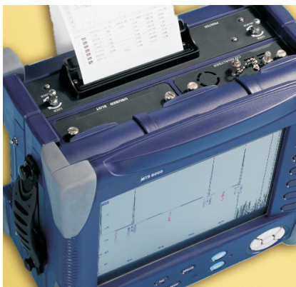
Internal printer with launch cable
