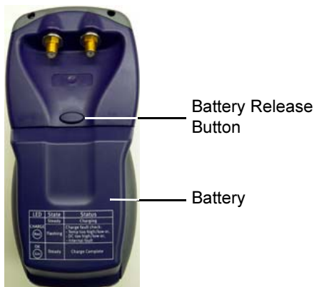
Figure 1 Back of DSAM Meter
