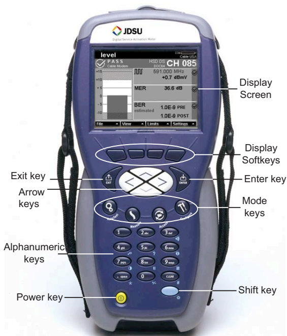
Figure 4 DSAM Meter Front Panel
