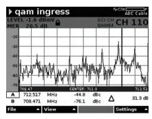
QAM Ingress test allows the technician to see what is going on underneath a live digital carrier which is usually not viewable due to the presence of the "havstack".
