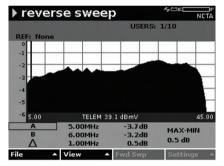
Tight reverse sweep points are setup in the sweep plan to view better resolution of the entire return path. Helping to find mismatches or other problems heading back to the headend or hubsite.
