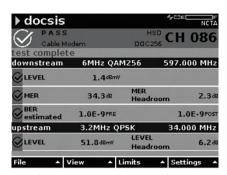
Using the range screen a technician is able to see what levels the DSAM's cable modem is reading and transmitting. This allows the tech to see how close the customer's cable modem would be to failing.
