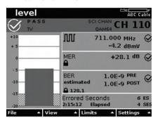
In the level mode on a digital channel, the signal's level and MER are measured and the channel's BER and errored seconds are tracked.
