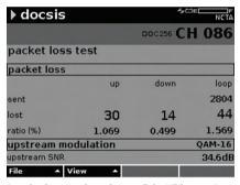
A packet loss test shows how well the HFC transmits RTP data packets. Using TruPacket SNMP community strings the DSAM is able to view both the up and down stream packet losses separately as well as the SNR the CMTS is receiving.
