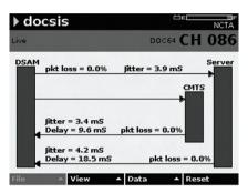
VoIPCheck is a voice quality verification test that runs over the DSAM's cable modem DOCSIS connection. It allows for segmentation between HFC and IP issues by showing on which side of the CMTS data impairments are present.
