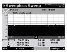
Sweepless Sweep provides a quick method to check cable system integrity using active channels to sweep the forward path. Sweep points do not need to be added and no forward path headend gear required.
