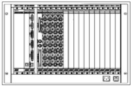
▲ Back view schematic of HCU1500 with four RPM1000 modules.
