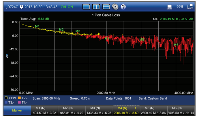
1-Port Cable Loss
