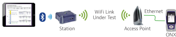
OneExpert supports the Wifi Advisor Dual-ended mode of operation providing TrueMargin and allows optimization of the Access Point placement
