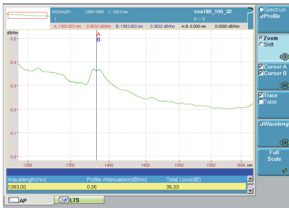
Figure 4: A spectral attenuation profile showing a loss vs. wavelength measurement
